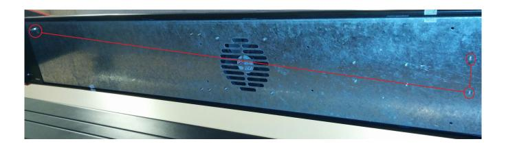
Now with the two screws on the right side are bridged and a length a wire is run from one of the bridged screws as shown above it is now time to run a wire from the grounding screw to the vinyl rollers on the stand.
