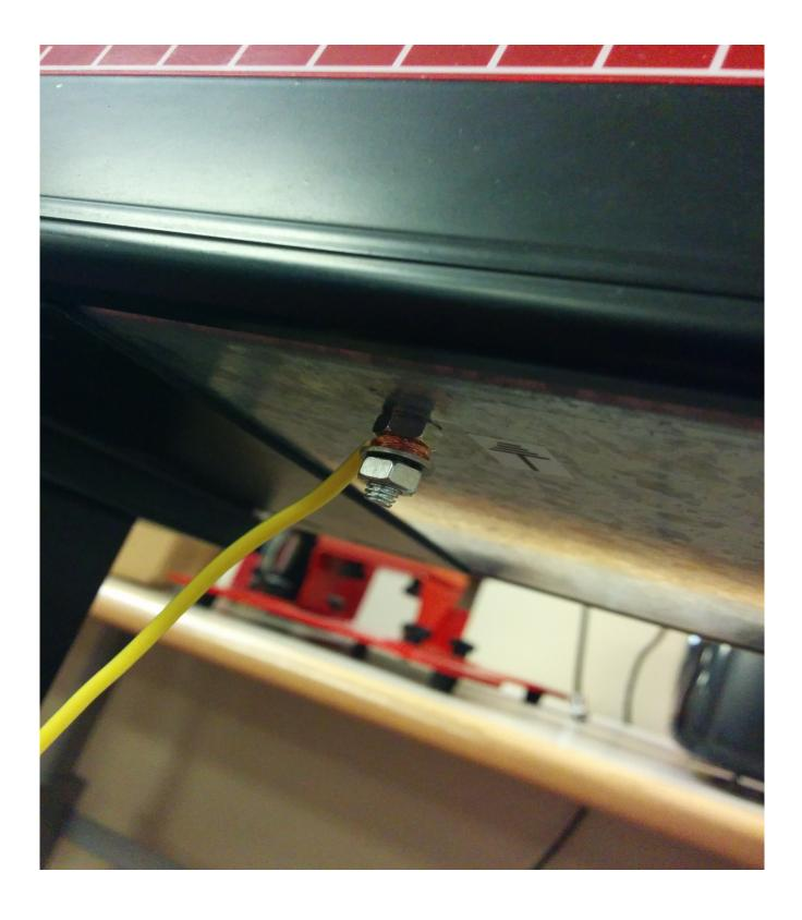
So now you should have all the grounds going to the grounding screw. Now we will run one more wire from the grounding screw to the electrical outlet cover screw as circled in red in the picture below.
