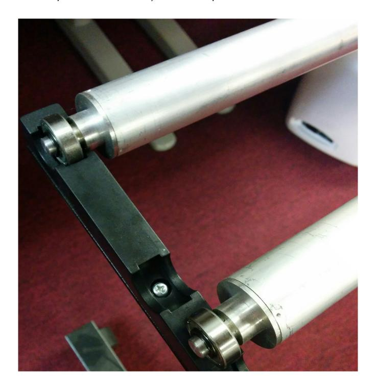
Now take your stripped wire and stick it into the groove and them put the vinyl roller back on top. The weight of the roller will hold the wire in place.
