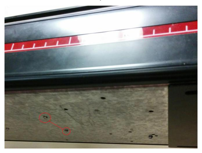
As you can see in the pictures I have run a line in between the screws. This is because you will need to run a length of wire between the two screws bridging them. Then from one of the bridged screws run another length of wire to the grounding screw located at the far left end on the bottom of the cutter.
